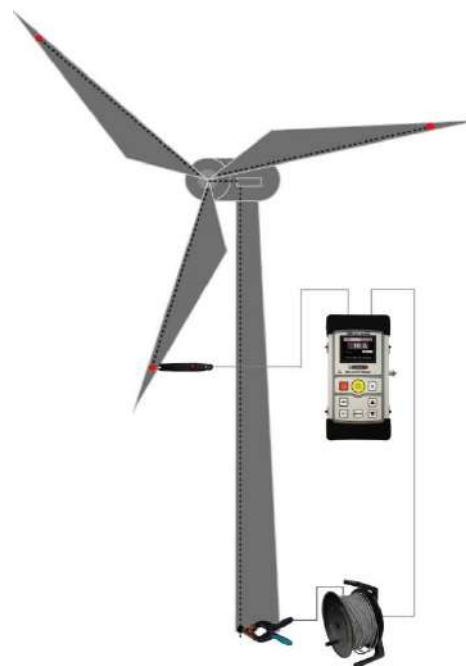
Lightning protection system testing with RMO-EH
