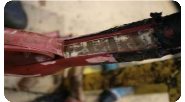
PD traces in a dry paper cable
