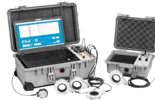
↑ In combination with the iPD transponder, Iona accurately and reliably locates PD.
