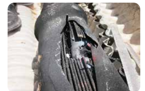
↙ Cable fault on paper-insulated mass-impregnated cable
