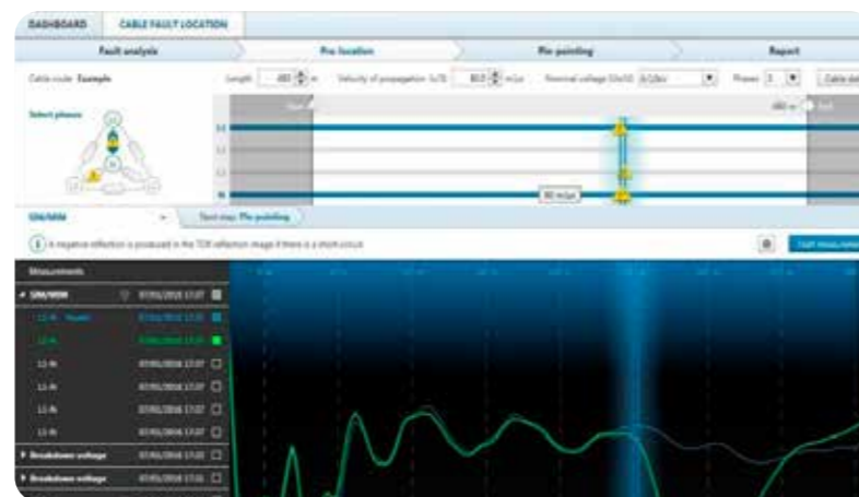
The BAUR Software 4 display enables clear visualisation of all important settings, fault location parameters, and cable data. The bottom part of the screen shows the measurement results and allows important events to be logged straight away.
