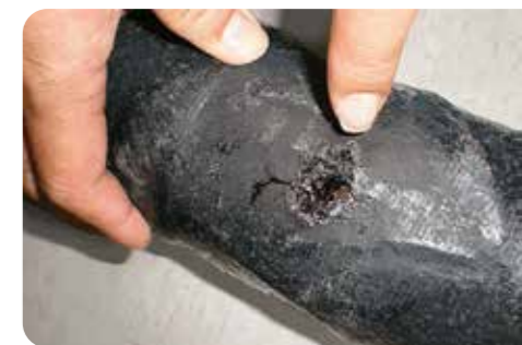
↙ Cable fault on paper-insulated mass-impregnated cable
