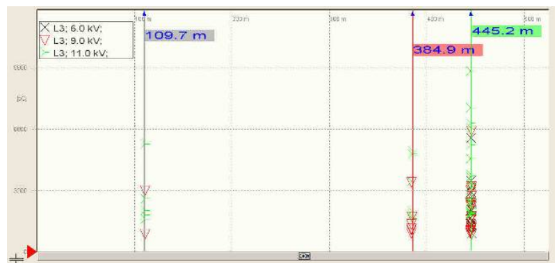
Figure 74 PD Localization Graph of a XLPE cable with 3 joints with PD activity
