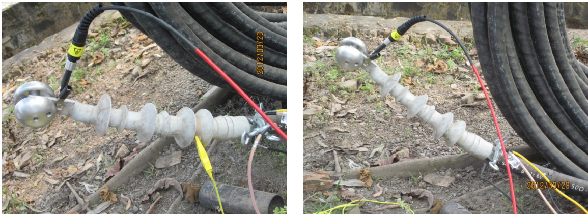
Figure 63, connection arrangement with guard ring and corona hoods (left), without guard ring (right); relative humidity 80%, 30°C
