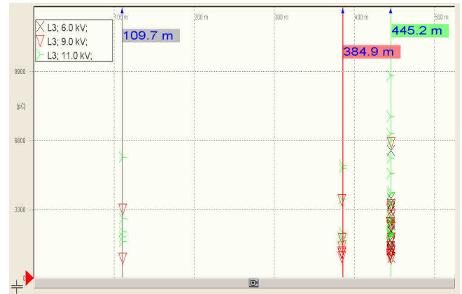
Figure 90 PD graph of XLPE cable with PD activity concentrated at 3 joints
