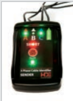
LED lights indicating connected and shorted phases
