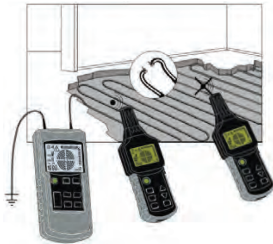
Detects breakers in radiant heating systems
