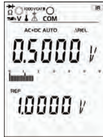
ΔREL MODE Displays relative values with respect to referenced measured value
