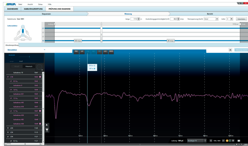
Figure 5: An example of the display during partial discharge measurement
