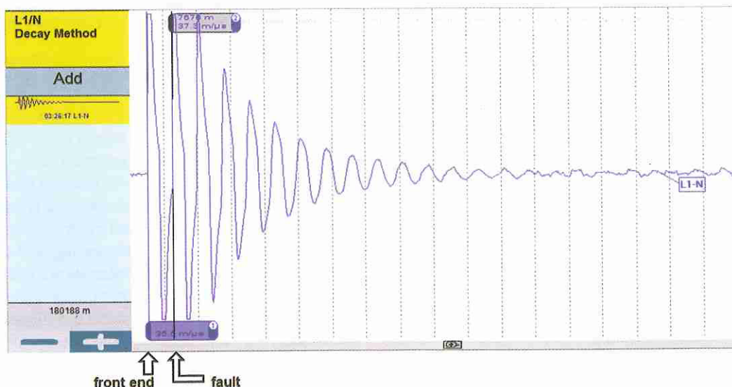
Figure 18. Decay method echogram revealing a 10-kV breakdown voltage intermittent fault at 7,586 m of distance from the front end of the cable [10].
