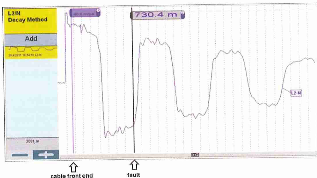
Figure 11. Echogram of the decay method applied to an AC cross-linked polyethylene-insulated submarine cable with an intermittent fault at 730.4 m [10].
