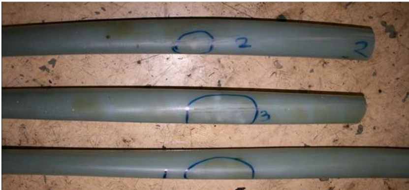
Visible white spots after removal of semi conductive layer, section #1, 2, 3
