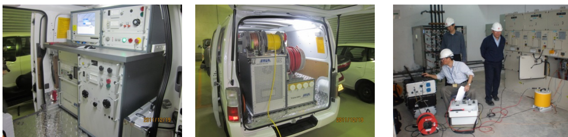
Figure 108: BAUR VLF TD / PD Systems used
