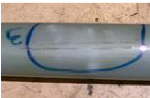
Dissection of water tree spot section #3
