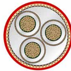
➤ Shielded concentric middle to high voltage cable, 3 conductors with own shield ea., faults between core and shield, core to core fault unlikely except for extreme external damage
