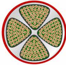
➤ Unshielded segmented low voltage cable 3 to 5 conductors, faults to ground and between cores.
