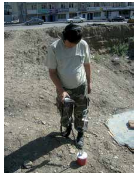
➤ field application acoustic fault location
