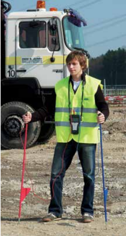
➤ step voltage method, two earth probes connected to UL30 receiver
