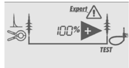
➤ KSG receiver display indicating direction, value, line conductivity
