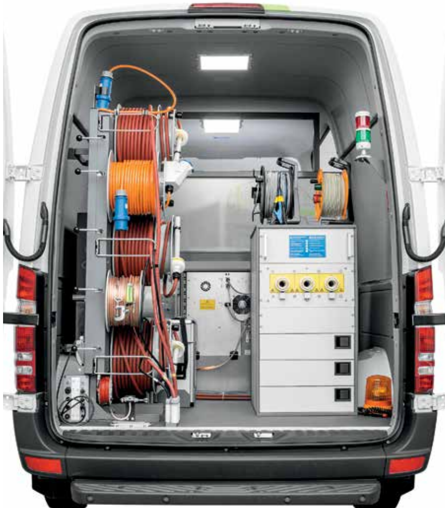
➤ Example of options in the high voltage area: motor-operated cable drum rack, external emergency stop unit and TDR connection cable
